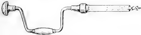
A Tube of Metal Fiber Placed Over the Bit Accelerates the Job
